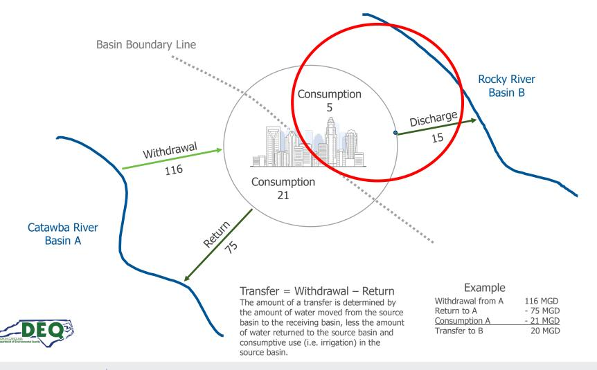
An IBT is a withdrawal, diversion or pumping of water from one source river basin to another river basin. The water from the source basin is treated and distributed to customers for everyday water usage, then collected and treated at wastewater treat ment plants before
